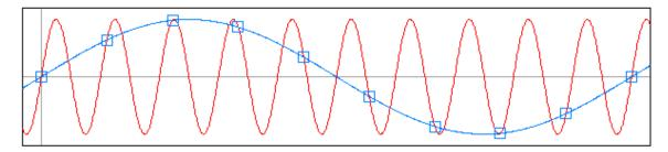
**Red:** actual signal **Blue**: received signal due to low frequency of observation
