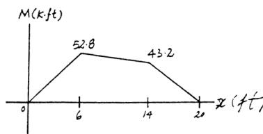
**\*11-24.** The beam has a flange width  $b = 8 \text{ in.}$  If the maximum bending stress is not to exceed  $\sigma_{\text{allow}} = 22 \text{ ksi}$ , determine the greatest weight of the machine that the beam can support. The center of gravity for the machine is at  $G$ , and the supports at  $B$  and  $C$  are smooth.
