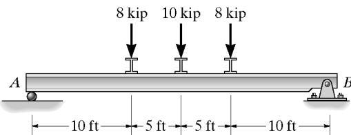
**Bending Stress:** From the moment diagram,  $M_{\max} = 155 \text{ kip}\cdot\text{ft}$ . Assume bending controls the design. Applying the flexure formula,
