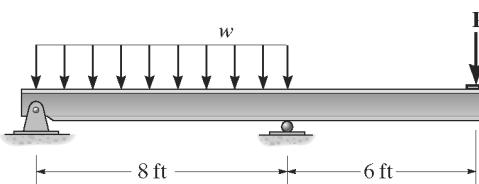
**Bending Stress:** From the moment diagram,  $M_{\text{max}} = 34.17 \text{ kip}\cdot\text{ft}$ . Assume bending controls the design. Applying the flexure formula.
