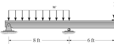
**Bending Stress:** From the moment diagram,  $M_{\max} = 60.0 \text{ kip}\cdot\text{ft}$ . Assume bending controls the design. Applying the flexure formula,
