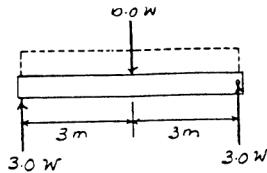
**Bending Stress:** From the moment diagram,  $M_{\max} = 4.50w$ .
