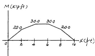
**11–5.** The simply supported beam is made of timber that has an allowable bending stress of  $\sigma_{\text{allow}} = 960 \text{ psi}$  and an allowable shear stress of  $\tau_{\text{allow}} = 75 \text{ psi}$ . Determine its dimensions if it is to be rectangular and have a height-to-width ratio of 1.25.
