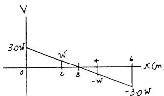
**Shear Stress:** Provide a shear stress check using the shear formula. From the shear diagram,  $V_{\max} = 3.00w = 10.01 \text{ kN}$ .
