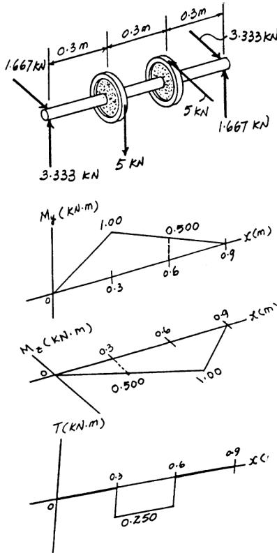
**11-39.** Solve Prob. 11-38 using the maximum-distortion-energy theory of failure with  $\sigma_{\text{allow}} = 180 \text{ MPa}$ .
