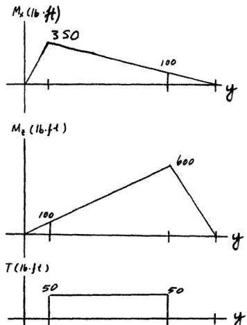
11-43 Solve Prob. 11-42 using the maximum-distortion-energy theory of failure,  $\sigma_{\text{allow}} = 20 \text{ ksi}$ .
