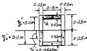
**Shear Flow:** Since there are two rows of nails, the allowable shear
