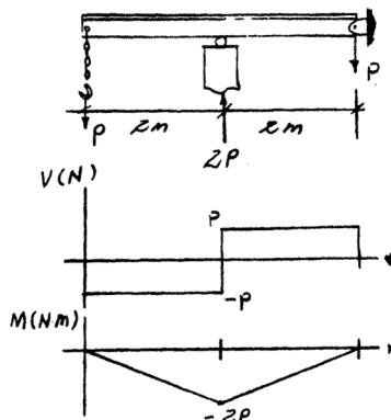
**11-22.** The timber beam has a rectangular cross section. If the width of the beam is 6 in., determine its height  $h$  so that it simultaneously reaches its allowable bending stress of  $\sigma_{\text{allow}} = 1.50 \text{ ksi}$  and an allowable shear stress of  $\tau_{\text{allow}} = 50 \text{ psi}$ . Also, what is the maximum load  $P$  that the beam can then support?
