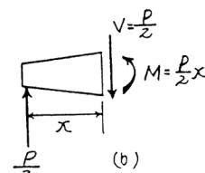
**Bending Stress:** Applying the flexure formula.
