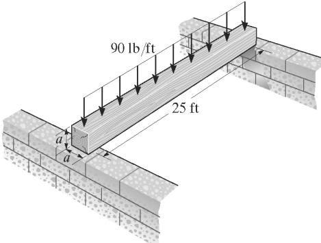
**Bending Stress:** From the moment diagram,  $M_{\max} = 7031.25 \text{ lb}\cdot\text{ft}$ . Assume bending controls the design. Applying the flexure formula,
