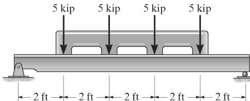
**Bending Stress:** From the moment diagram,  $M_{\max} = 30.0 \text{ kip} \cdot \text{ft}$ . Assume bending controls the design. Applying the flexure formula.
