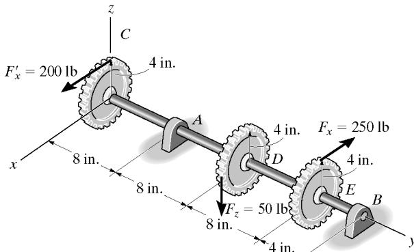
**Shaft Design:** By observation, the critical section is located at support A, where  $M = \sqrt{1600^2 + 0} = 1600 \text{ lb} \cdot \text{in}$  and  $T = 800 \text{ lb} \cdot \text{in}$ . Using the maximum shear stress theory,
