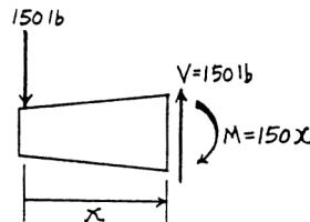
**Bending Stress:** Applying the flexure formula.
