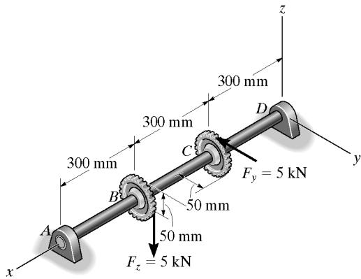
**Shaft Design:** By observation, the critical section is located just to the left of gear *C* and just to right of gear *B*, where  $M = \sqrt{1.00^2 + 0.500^2} = 1.118 \text{ kN} \cdot \text{m}$  and  $T = 0.250 \text{ kN} \cdot \text{m}$ . Using the maximum shear stress theory.
