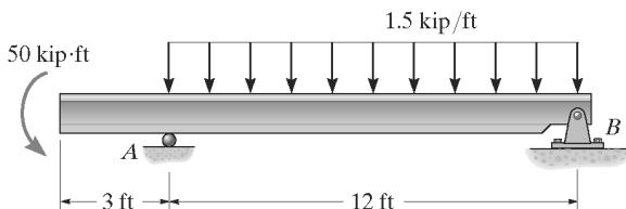
**Bending Stress:** From the moment diagram,  $M_{\max} = 50.0 \text{ kip}\cdot\text{ft}$ .
