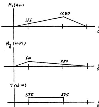
**\*11-56.** The bearings at *A* and *B* exert only *x* and *z* components of force on the steel shaft. Determine the shaft's diameter to the nearest millimeter so that it can resist the loadings of the gears without exceeding an allowable shear stress of  $\tau_{\text{allow}} = 80 \text{ MPa}$ . Use the maximum-distortion-energy theory of failure with  $\sigma_{\text{allow}} = 200 \text{ MPa}$ .
