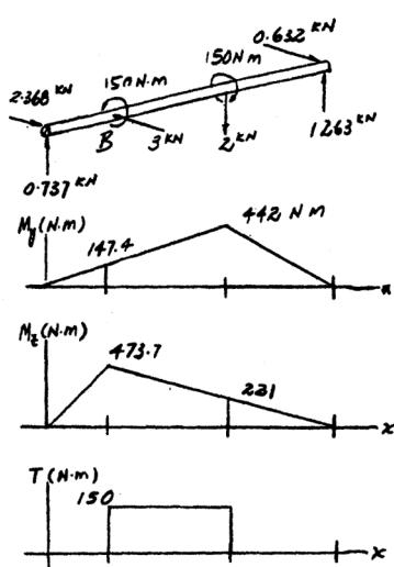
**11-41.** Solve Prob. 11-40 using the maximum-distortion-energy theory of failure.  $\sigma_{\text{allow}} = 130 \text{ MPa}$ .
