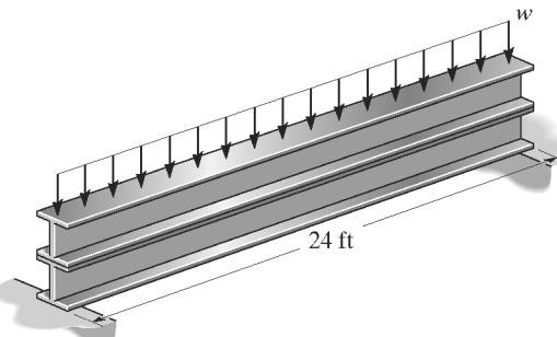
**Section properties:** For W12 x 22 ( $d = 12.31 \text{ in.}$ ,  $I_x = 156 \text{ in}^4$ ,  $t_w = 0.260 \text{ in.}$ ,  $A = 6.48 \text{ in}^2$ )
