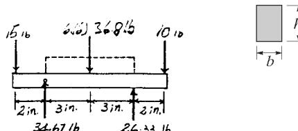
**Bending Stress:** From the moment diagram,  $M_{\text{max}} = 30.0 \text{ lb} \cdot \text{in}$ . Assume bending controls the design. Applying the flexure formula.
