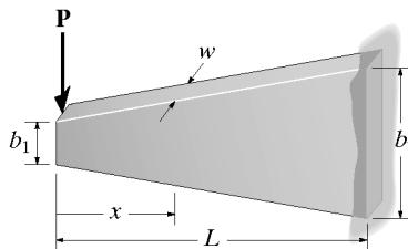
$$\frac{b - b_1}{x} = \frac{b_2 - b_1}{L} \quad b = \frac{x(b_2 - b_1) + b_1 L}{L}$$
