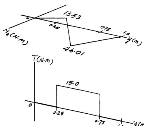
**11-45.** The shaft is supported on journal bearings that do not offer resistance to axial load. If the allowable shear stress for the shaft is  $\tau_{\text{allow}} = 35 \text{ MPa}$ , determine to the nearest millimeter the smallest diameter of the shaft that will support the loading. Use the maximum-shear-stress theory of failure.
