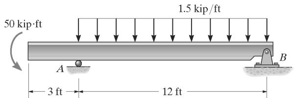
**Bending Stress:** From the moment diagram,  $M_{\max} = 50.0 \text{ kip}\cdot\text{ft}$ . Assume bending controls the design. Applying the flexure formula,
