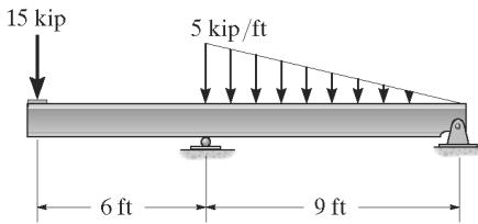
**Bending Stress:** From the moment diagram,  $M_{\max} = 90.0 \text{ kip} \cdot \text{ft}$ . Assume bending controls the design. Applying the flexure formula.
