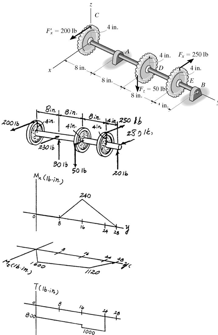
**11-47.** Solve Prob. 11-46 using the maximum-shear-stress theory of failure with  $\tau_{\text{allow}} = 6 \text{ ksi}$ .
