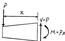
**Bending Stress:** Applying the flexure formula.
