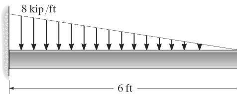
**Bending Stress:** From the moment diagram,  $M_{\max} = 48.0 \text{ kip} \cdot \text{ft}$ . Assume bending controls the design. Applying the flexure formula.
