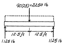
**Shear Stress:** Provide a shear stress check using the shear formula
