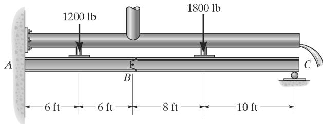
**Bending Stress:** From the moment diagram,  $M_{\max} = 19.2 \text{ kip}\cdot\text{ft}$  for member *AB*. Assuming bending controls the design, applying the flexure formula.
