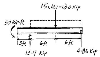
**\*11-20.** The compound beam is made from two sections, which are pinned together at *B*. Use Appendix B and select the light wide-flange beam that would be safe for each section if the allowable bending stress is  $\sigma_{\text{allow}} = 24 \text{ ksi}$  and the allowable shear stress is  $\tau_{\text{allow}} = 14 \text{ ksi}$ . The beam supports a pipe loading of 1200 lb and 1800 lb as shown.
