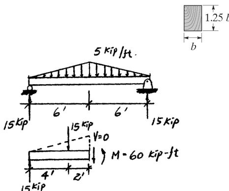
**11–6.** The wooden beam has a rectangular cross section and is used to support a load of 1200 lb. If the allowable bending stress is  $\sigma_{\text{allow}} = 2 \text{ ksi}$  and the allowable shear stress is  $\tau_{\text{allow}} = 750 \text{ psi}$ , determine the height  $h$  of the cross section to the nearest  $\frac{1}{4} \text{ in.}$  if it is to be rectangular and have a width of  $b = 3 \text{ in.}$  Assume the supports at  $A$  and  $B$  only exert vertical reactions on the beam.
