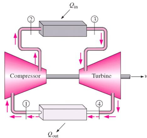
**9-94** A simple ideal Brayton cycle with air as the working fluid operates between the specified temperature and pressure limits. The net work and the thermal efficiency are to be determined.
