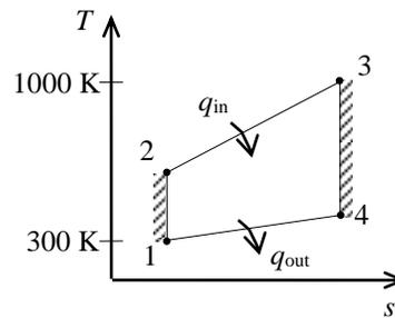
Applying the first law to the constant-pressure heat addition process 2-3 produces
