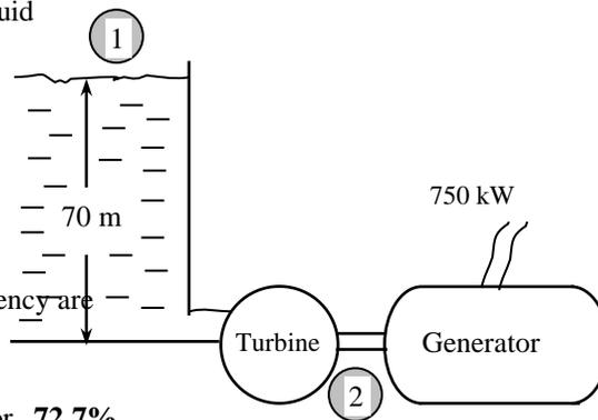
Therefore, the reservoir supplies 1031 kW of mechanical energy to the turbine, which converts 800 kW of it to shaft work that drives the generator, which generates 750 kW of electric power.
