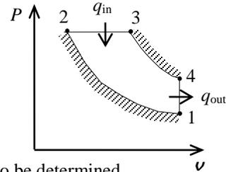
**9-57** An ideal diesel cycle has a cutoff ratio of 1.2. The power produced is to be determined.
