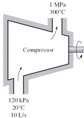
**Solution (5-51)** Air is compressed at a rate of 10 L/s by a compressor. The work required per unit mass and the power required are to be determined.
