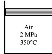
**Solution (4-25)** A piston-cylinder device contains air gas at a specified state. The air undergoes a cycle with three processes. The boundary work for each process and the net work of the cycle are to be determined.
