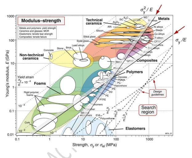
Let us consider the material index concept for the selection of the best material for an *elastic hinge.* For this you need the equation linking the maximum filament strength as a function of the radius of curvature R, the thickness t, and the Young's modulus of the material.
