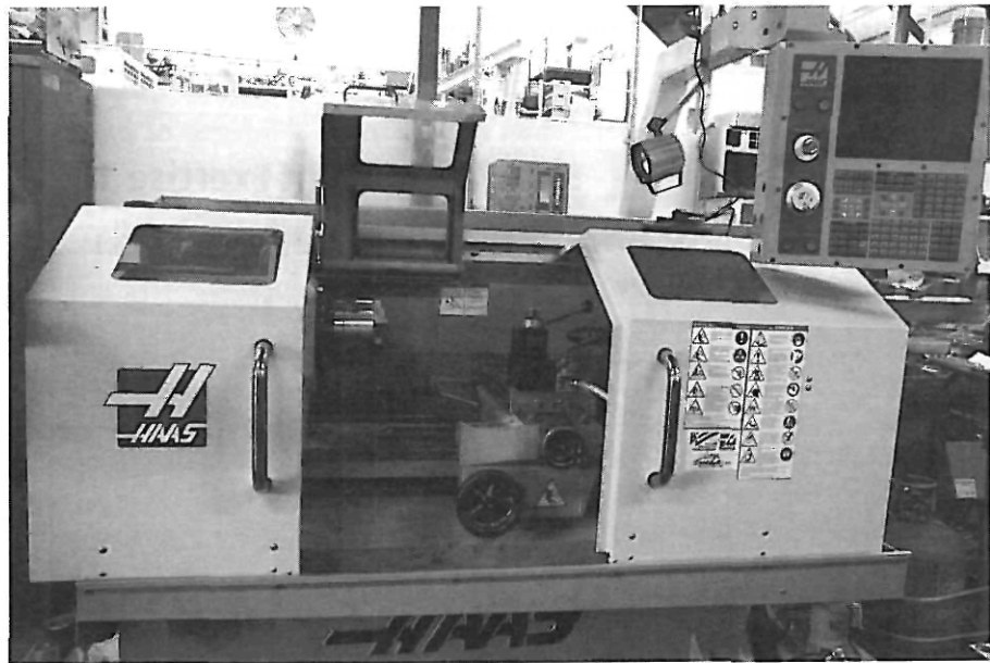
FIGURE 13.12 A lathe using digital numerical control (© David J. Green—Industry/Alamy)
