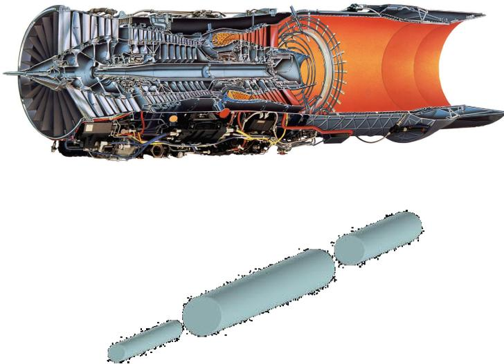
Figure 3.2: Engine beam model [Courtesy of [www.milnet.com](http://www.milnet.com)]
