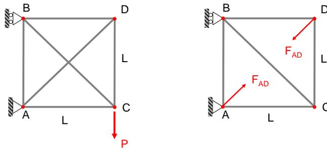
Figure 8.3: Statically indeterminate six bar truss
