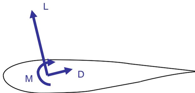
Figure 5.4: Combined airfoil load
