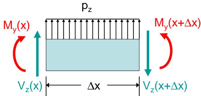
Figure 3.5: Infinitesimal beam segment
