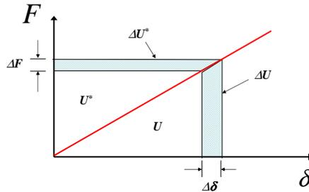
Figure 6.3: Linear force-displacement diagram
