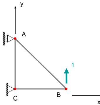
Figure 6.4: Truss structure with applied dummy load
