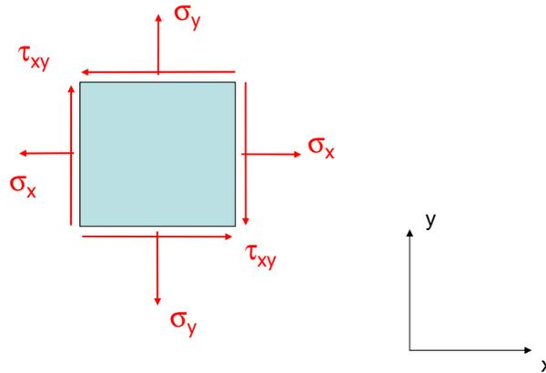
Figure 4.2: Example of fully loaded stress element
