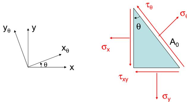
Figure 4.3: Free body diagram for the plate equilibrium equations
