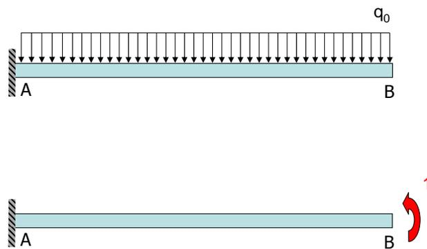
Figure 7.1: Statically determinate beam example
