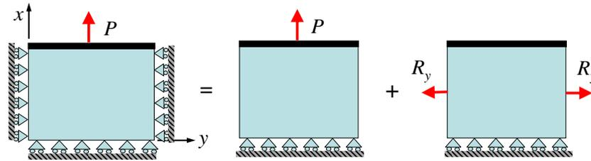
Figure 10.1: Biaxial stress state plate
