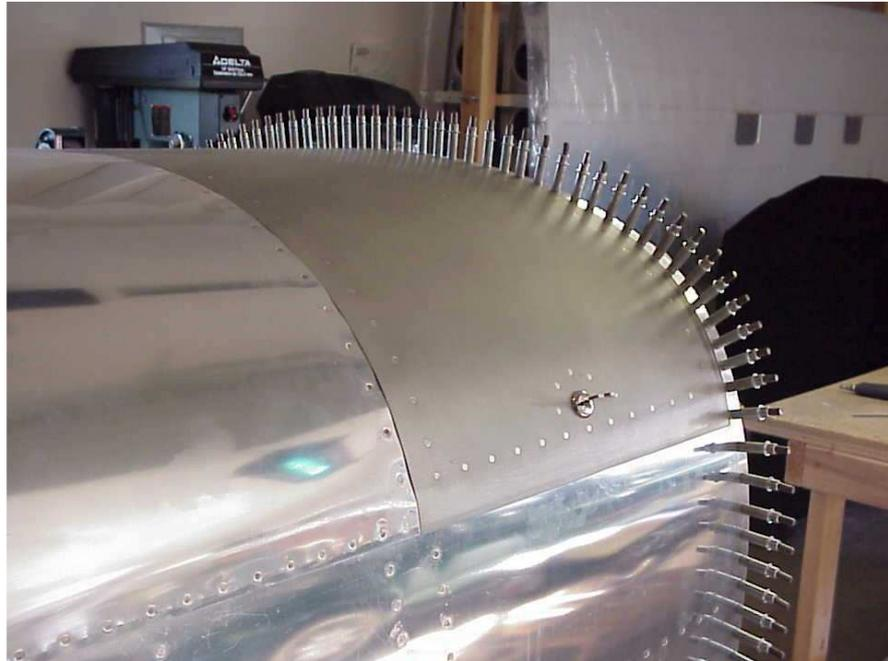
Figure 4.1: Example of an aircraft riveted plate skin [Courtesy of [www.romeolima.com](http://www.romeolima.com)]
