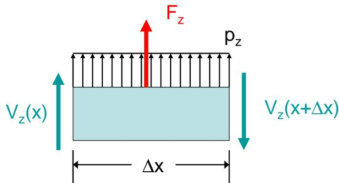
Figure 3.6: Force jump over an infinitesimal beam segment
