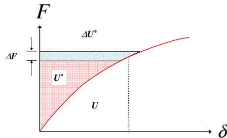
Figure 6.2: Principle of complementary energy
