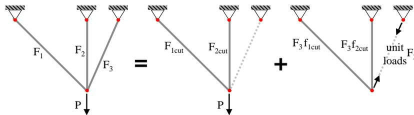
Figure 8.2: Split-up of an indeterminate truss
