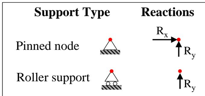
Figure 2.3: Truss support types
