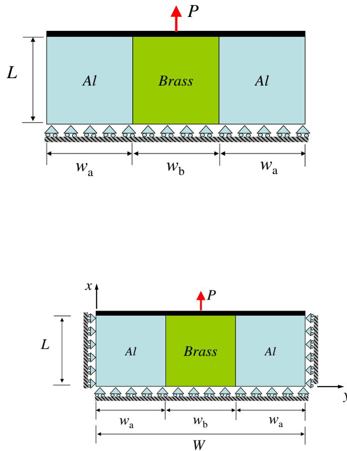
Figure 10.2: Indeterminate multilayered plates (left: one statically indeterminate force, right: two statically indeterminate forces)
