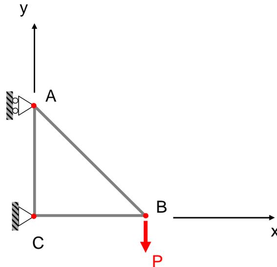
Figure 2.6: Three bar truss example
