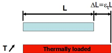
Figure 11.1: Thermal extension of a bar
