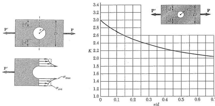
Figure 5.2: Geometric definitions and  $K$  factor for a hole [Courtesy of Beer, P.F., *Mechanics of Materials*]
