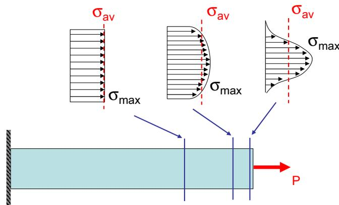
Figure 5.1: Illustration of the principle of De Saint-Venant
