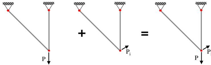
Figure 8.1: Force superposition principle
