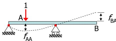
Figure 9.1: Illustration of the flexibility coefficient
