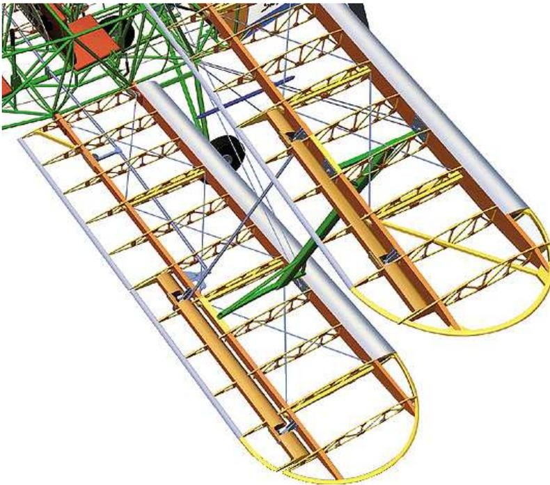
Figure 2.1: Rib truss structure example [Courtesy of [www.steenaero.com](http://www.steenaero.com)]
