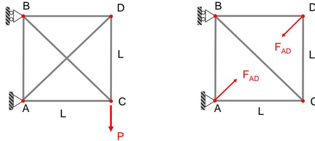
Figure 11.3: Statically indeterminate six bar truss
