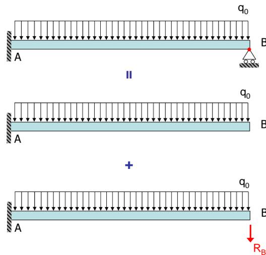
Figure 9.3: Analysis example of a statically indeterminate beam
