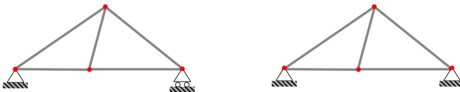
Figure 2.4: Statically determinate and indeterminate trusses
