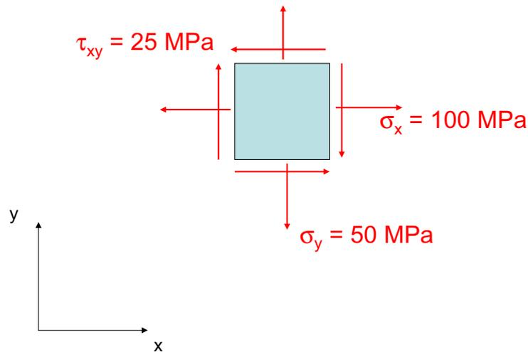
Figure 4.6: Example load case on a stress element
