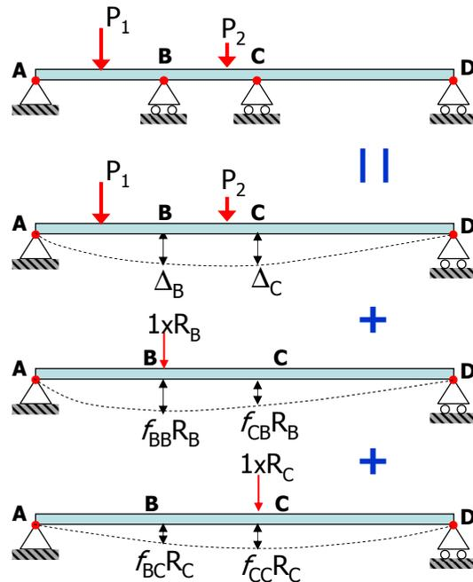
Figure 9.2: Solution of a statically indeterminate beam using flexibility coefficients
