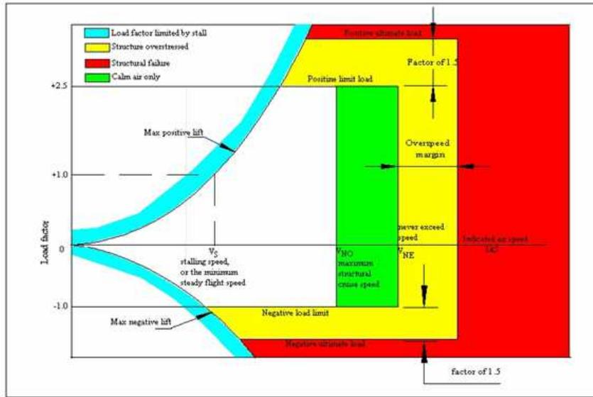
Figure 5.5: Flight envelope containing multiple load cases
