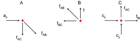
Figure 6.5: Nodal internal dummy loads
