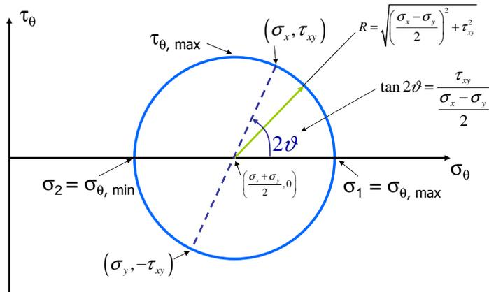
Figure 4.4: Layout and definition of Mohr's circle
