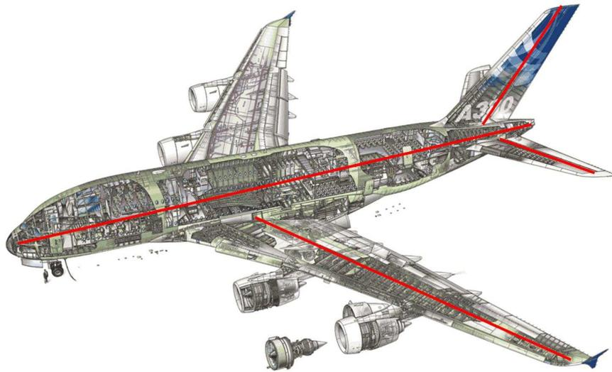
Figure 3.1: Aircraft beam model [Courtesy of [www.flightinternational.com](http://www.flightinternational.com)]
