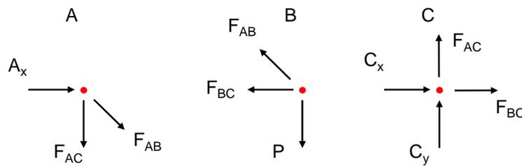
Figure 2.7: Free-body diagram of each node
