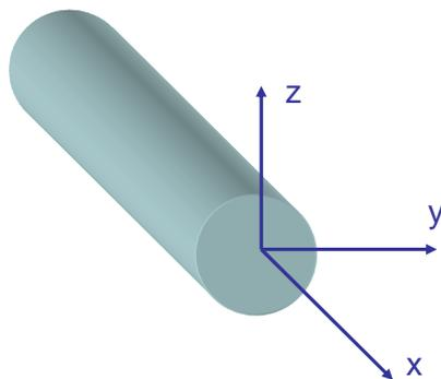
Figure 3.3: Local beam axes
