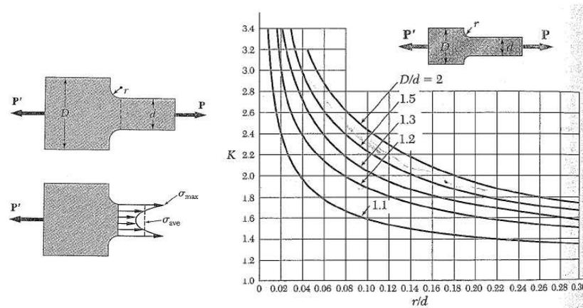
Figure 5.3: Geometric definitions and  $K$  factor for a cross-section change [Courtesy of Beer, P.F., *Mechanics of Materials*]
