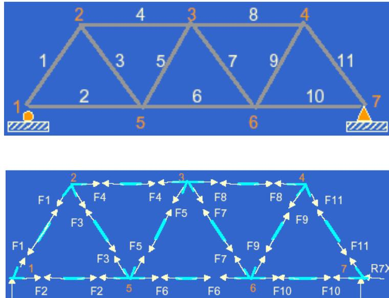
Figure 2.5: Internal force distribution inside a truss
