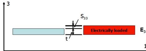
Figure 11.2: Piezoelectric thickness change of a bar
