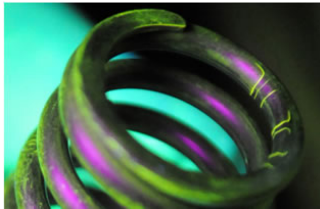
Figure 9.5 Principles of penetrant inspection
