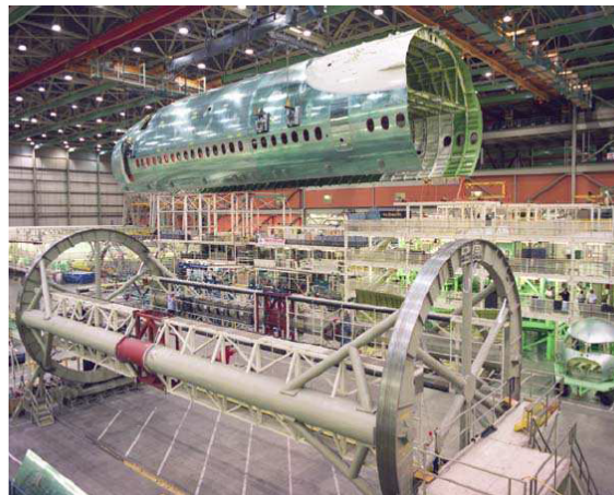
Figure 6.7. A rotational jig for a fuselage section
