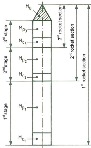
Figure 3.1: Nomenclature of a Multi-Stage rocket.
