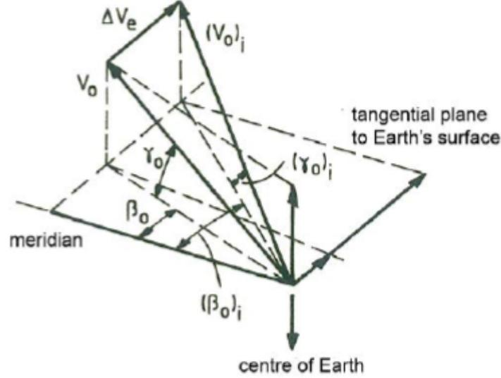
Figure 4.4: Transformation of local velocity and angles to inertial velocity and angles
