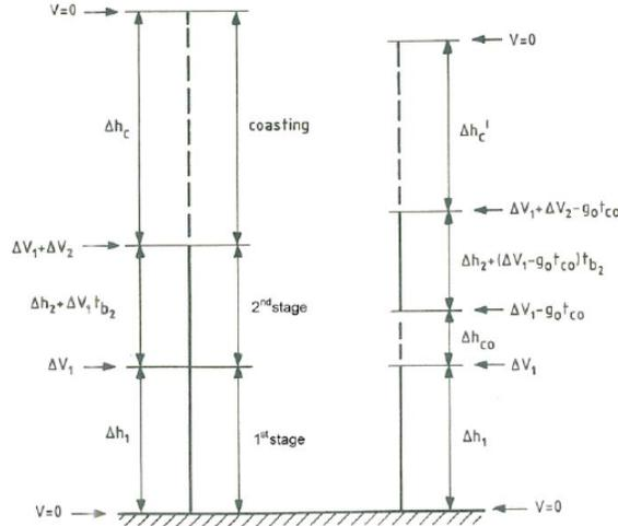
Figure 3.2: Vertical flight with and without coasting
