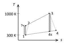
$w_{s,C,in} = h_{2s} - h_1 = c_p (T_{2s} - T_1) = (1.005 \text{ kJ/kg} \cdot \text{K})(610.2 - 300)\text{K} = 311.75 \text{ kJ/kg}$  $w_{s,T,out} = h_3 - h_{4s} = c_p (T_3 - T_{4s}) = (1.005 \text{ kJ/kg} \cdot \text{K})(1000 - 491.7)\text{K} = 510.84 \text{ kJ/kg}$
